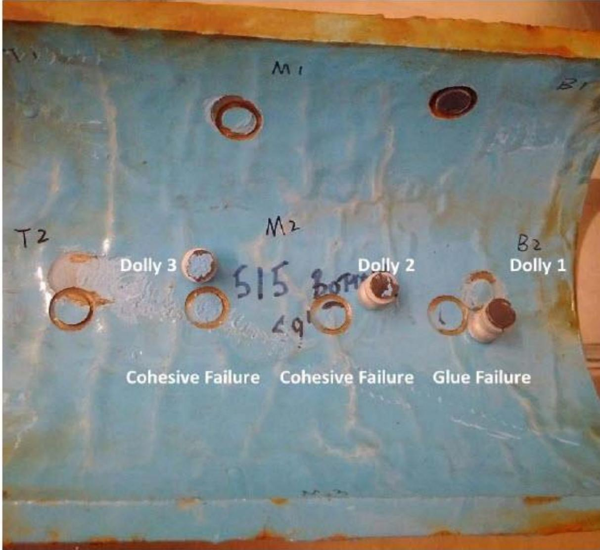
Figure 4: Adhesion testing of lining
