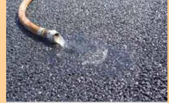
Figure 1. Porous asphalt allows water to flow through it. Photo courtesy of the National Asphalt Paving Association
