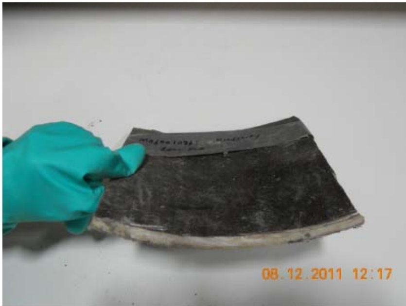
Figure 6: Kingsway and Richard CIPP Liners - sampled Dec 2011
