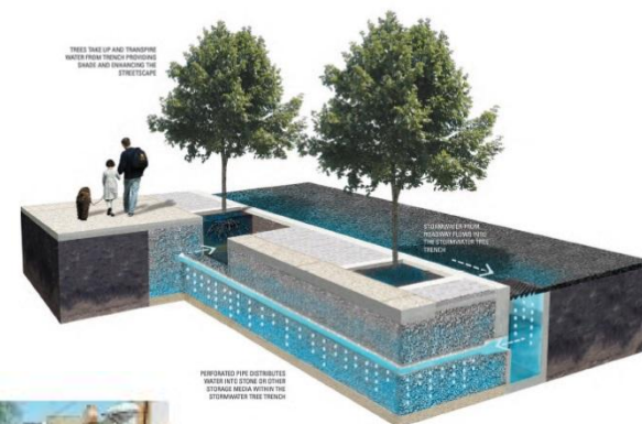
Figure 2.4: Three-Dimensional View of a Stormwater Tree Trench
