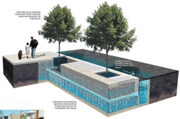
Figure 2.4: Three-Dimensional View of a Stormwater Tree Trench
